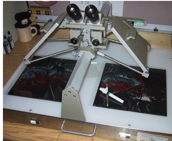
Figure 38. Stereoscope equipment used for photointerpreting color infrared aerial photographs.
