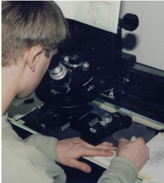
Figure 37. Stereoscope equipment used for photointerpreting true color aerial photographs.
