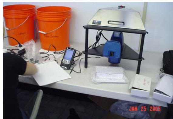
Figure 6-2. Innov-X XT400 XRF analyzer set up for bench-top analysis.
