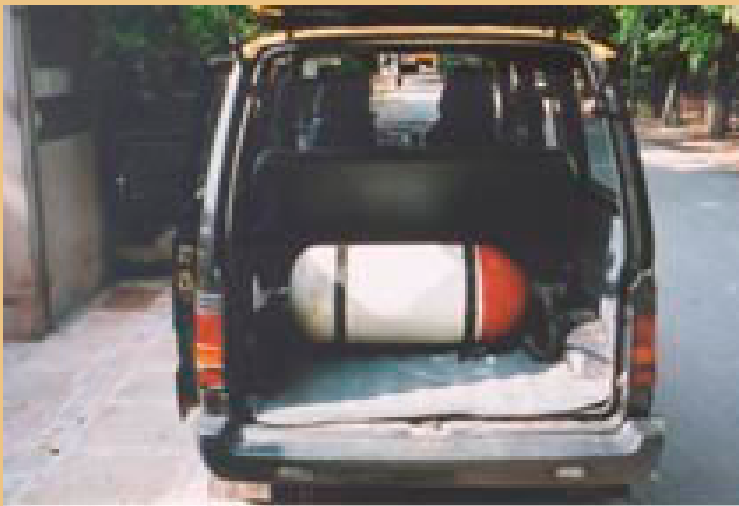
Compressed Natural Gas cylinder in a car.
