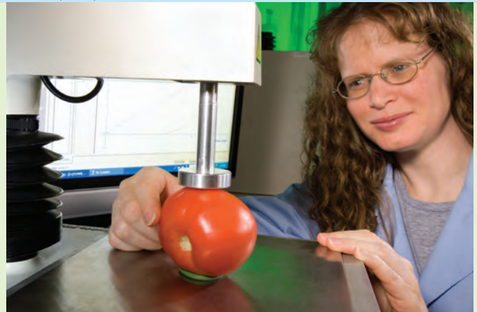
Technician Judith Dumm measures tomato firmness with compression tests.
