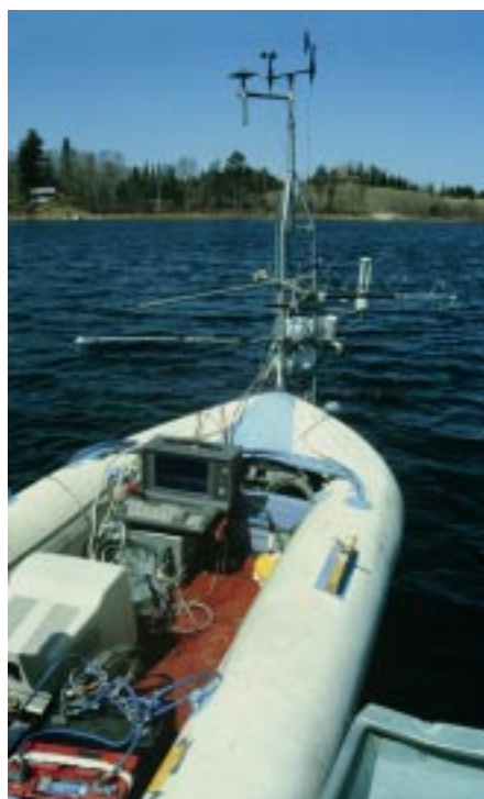
Figure 5. Measurement of evaporation and carbon flux using the eddy-correlation method requires a stable platform such as this tower installed near the center of Williams Lake.
