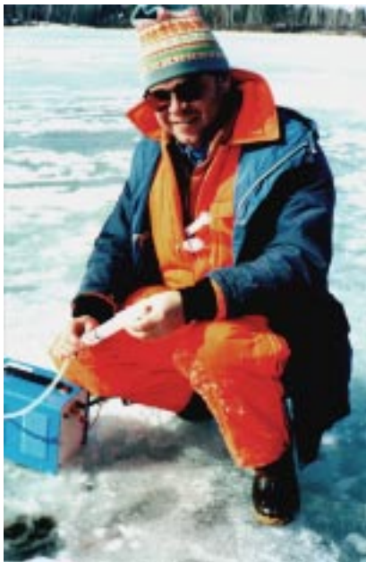
Figure 4. Collection of water sample through ice cover for determination of carbon dioxide and methane dissolved in the lake water.
