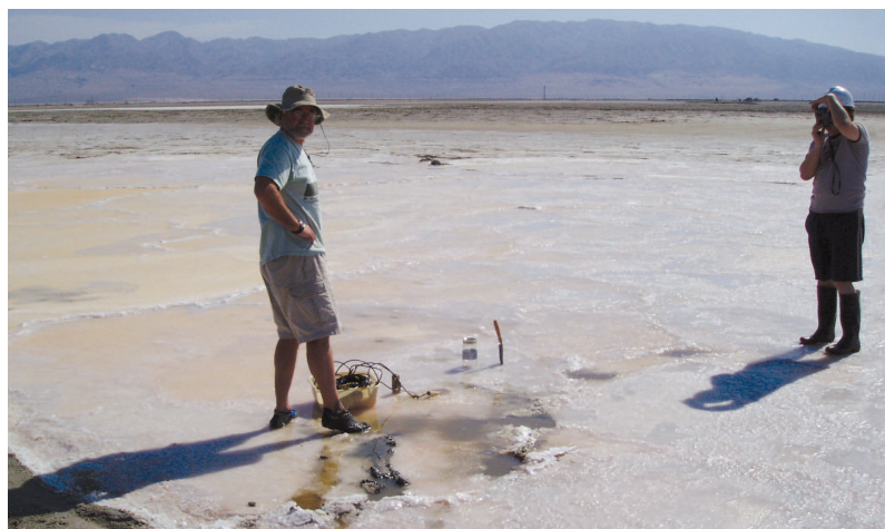
FIGURE 2B Collection of samples beneath the thick salt crust at Searles Lake. Searles Lake is an evaporated version of Mono Lake. USGS scientists Larry Miller (foreground) and Tom Kulp had to chip a hole through the thick (~6 cm) salt crust to access the underlying dense brine, about 5 cm deep, below which lay the anoxic sediments that they recovered by use of hand corers. PHOTO SHELLEY E. HOFFT, USGS
