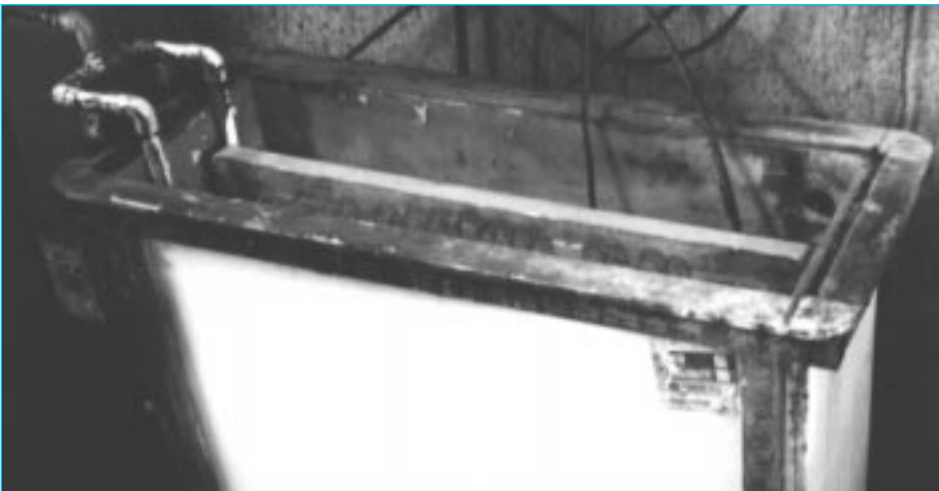
T.S. Designs' enclosed reclaim tank has cut the company's use of water in half.
