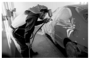
✤ By using a supplied-air, positive-pressure respirator, painters are much less likely to breathe harmful chemicals in paint spray. Most paint manufacturers say a supplied-air respirator is a Amust<sup>@</sup> when spraying highly toxic materials like isocyanates, the hardener in polyurethane clearcoats and in many primers. An air-purifying respirator will not provide adequate protection unless you develop and implement a proper filter change -out schedule, which can be a complex process.
