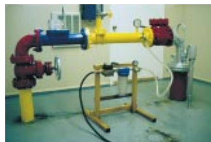
Virus sampling equipment and public water supply well.
