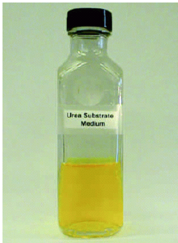
Photo 1. Urea Substrate Medium. After adjusting the pH of the medium to 3-4, the Urea Substrate Medium should be straw-yellow in color.
