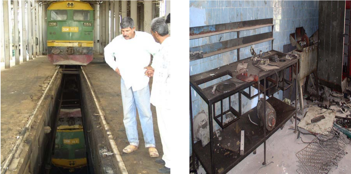
Figure 7. Flooded pit and forge (with empty equipment slots) in Al Basra shed
