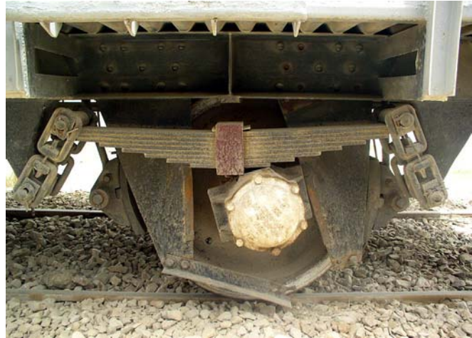
Broken Axle Assembly
