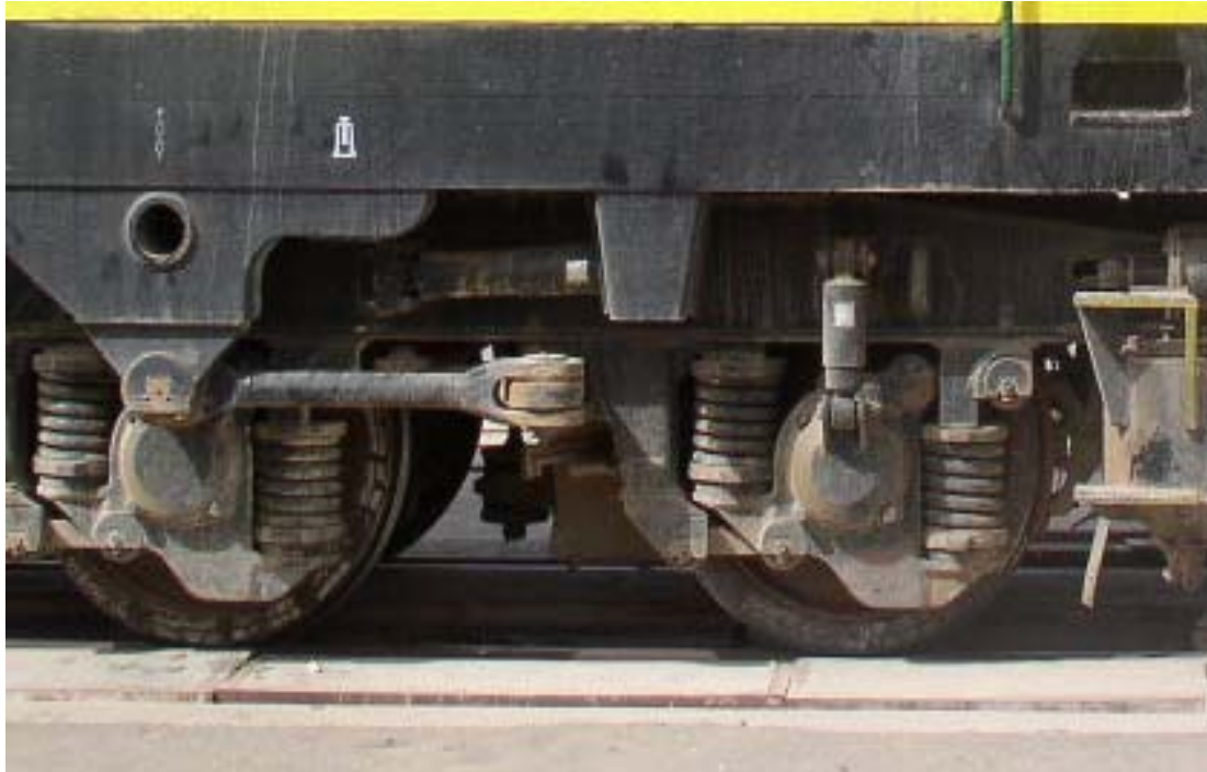
Figure 13. Locomotive brake block (to right of picture) taken just before departure on 550km journey. With no train brakes, this thin block, with others on the locomotive of similar quality, has to stop the whole train.
