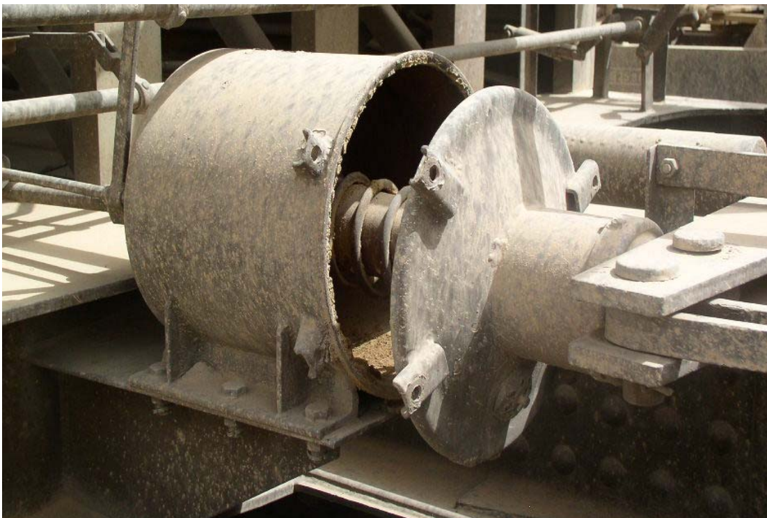
Figure 12. Brake piston on grain hopper (the majority of the hoppers were also missing distribution valves)
