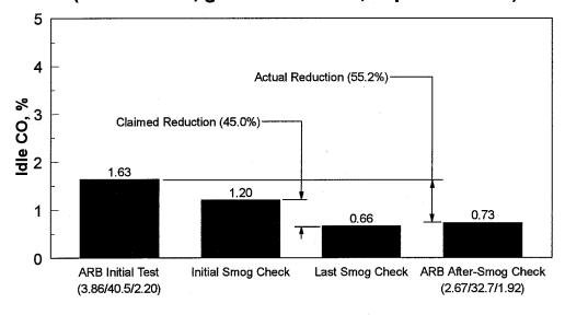
ARB After-Smog readings do not exceed Last Smog Check readings by more than 400 ppm/2.00%. 641 vehicles met the criteria.
