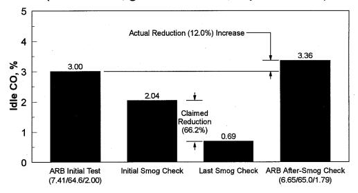
ARB After-Smog readings exceed Last Smog Check readings by at least 400 ppm HC or 2.00% CO. 190 vehicles met the criteria.
