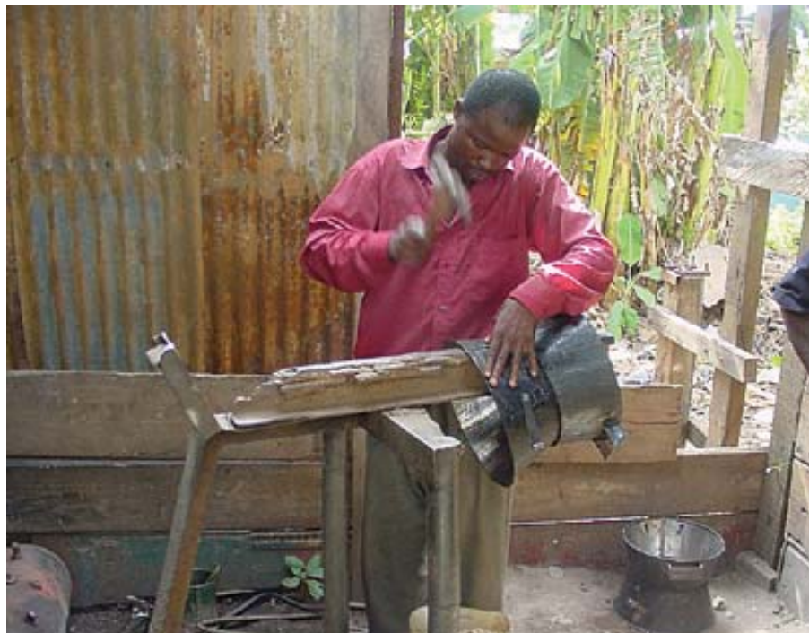
A trained artisan in Ghana crafts the shell for a ceramic-lined stove. These stoves reduce the amount of wood needed to cook food. USAID promotes the conservation of forests through this energy-saving device.
