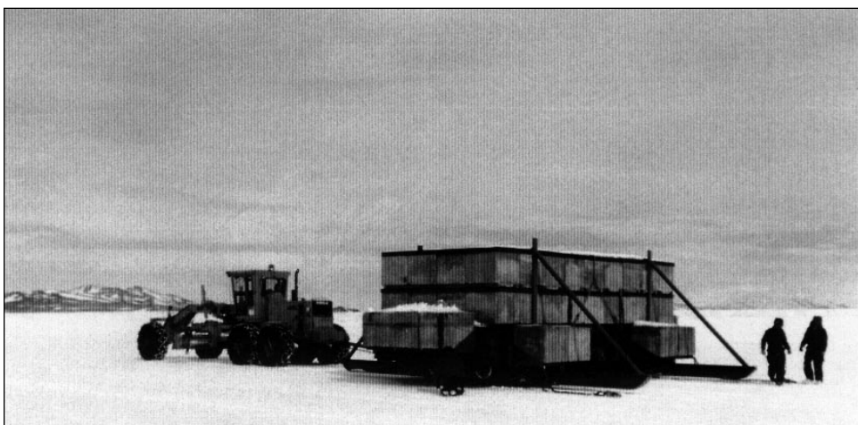
Figure 5. Proof cart configured and ballasted for C-141 aircraft proof testing.
