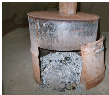
Figure 2. Representative of stoves used in 25 percent of homes surveyed, this stove was not designed to burn coal safely. Photograph by Veronica Francisco-Lapahie, Diné College, 2004; used with permission.
