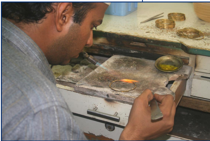
An artisan in a Karachi workshop solders gold bangles with a gas flame.
