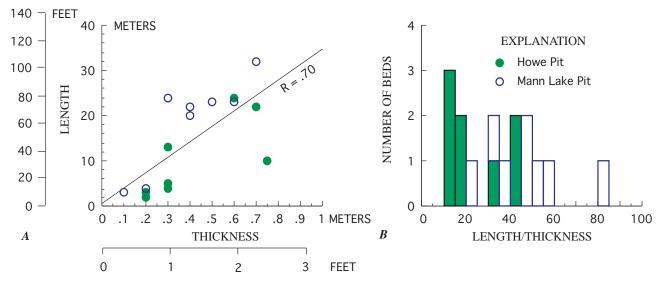
**Figure 2.**—Dimensions of clay lenses in the Howe and Mann Lake gravel pits: A) lens length (apparent, measured on pit face) versus maximum thickness; B) frequency distribution of lens length/thickness ratios of clay lenses.
