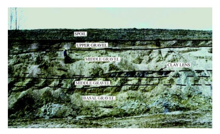
**Figure 1.**—Photograph showing clay lens in lower part of middle gravel unit, sampled for pollen and chemical analysis, Mann Lake pit. Location shown in Figure 7 of Part A.
