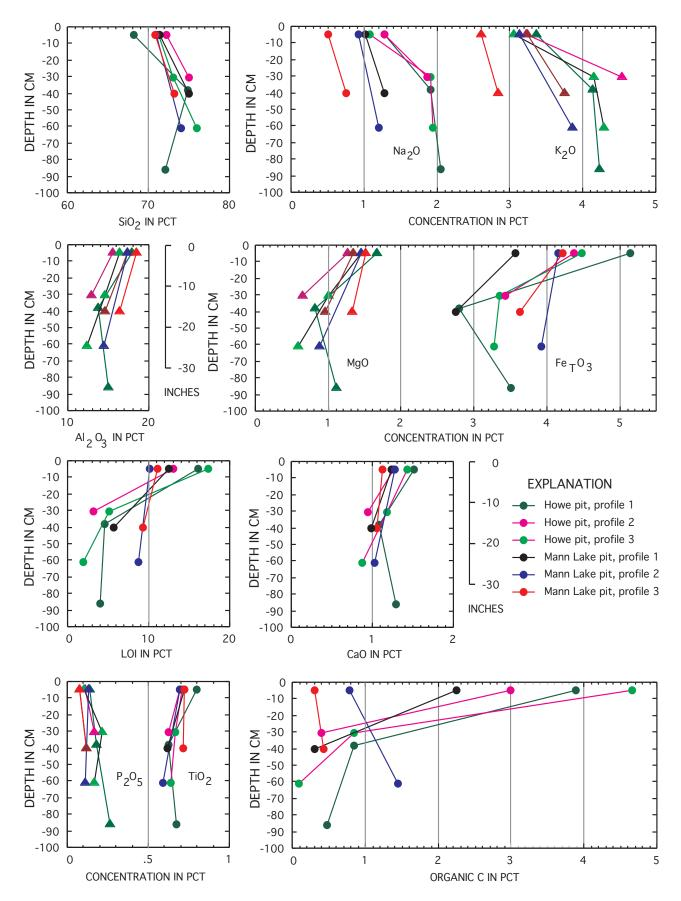
**Figure 4.**—Vertical profiles of major-element oxides, loss on ignition at 925°C, and organic carbon in six clay lenses from the Howe and Mann Lake pits. All major oxide values recalculated to volatile-free basis.
