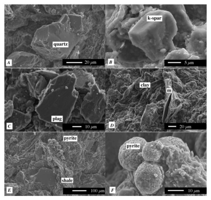
**Figure 3.**—Scanning electron microscope (SEM) photographs of individual mineral grains in clay lens, Howe pit. Most grains are silt size. A, quartz; B, potassium feldspar (k-spar); C, plagioclase (plag); D, probable illite (clay) and mica (m); E, shale fragment with small spheres of framboidal pyrite, probably derived from Cretaceous shale; and F, detail of framboidal pyrite in E. Scale bar in micrometers ( $\mu$ m); one  $\mu$ m = 10<sup>-6</sup> meter.
