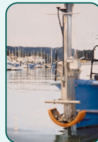
Photo of sonar equipment mounted to survey boat
