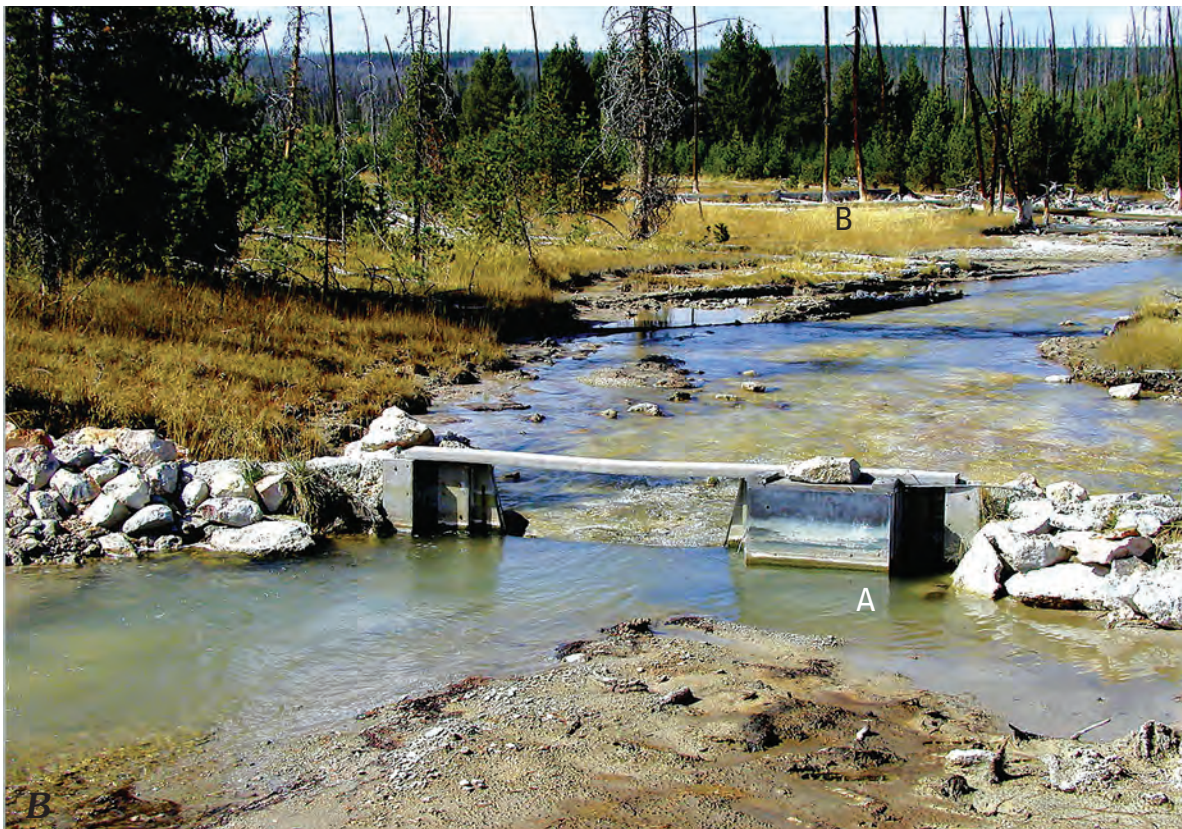
Figure 1. A , Photograph of weir looking upstream. B , Photograph of weir looking downstream. A , The gray plastic stilling well box can be seen at the right of the weir plate. B , Confluence of Tantalus Creek and Gibbon River is just out of sight beyond the upper left side of the photograph.
