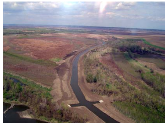
Aerial photo of Lower Hamburg Bend chute constructed by U.S. Army Corps of Engineers as part of the Missouri River Mitigation Program.
