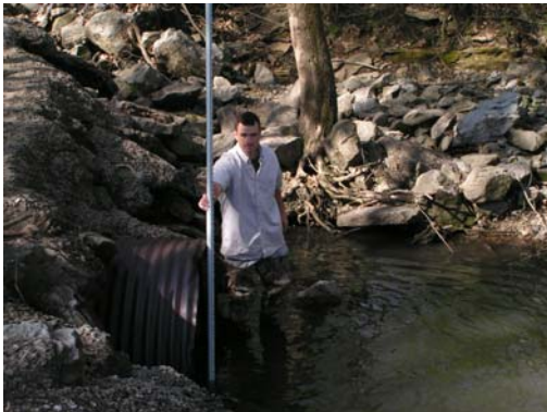
Nick Frohnauer measures culvert in low water crossing to assess fish passage.
