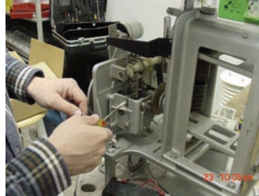
The inside of the old mechanical Fisher / Porter gage
