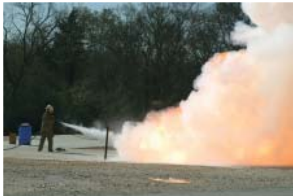
Figure 9 The preferred fire extinguishing agent for LNG is dry chemical, potassium bicarbonate.
