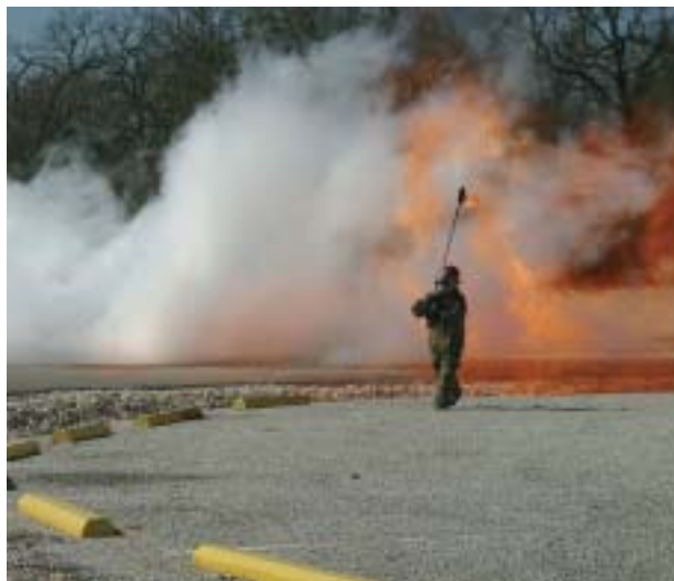
Figure 8 If an ignition source is encountered, LNG vapors will ignite and burn back to the origin of the spill. In this demonstration at Texas A&M, the LNG is ignited and slowly burns back to the source.
