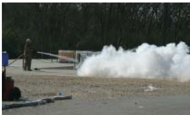
Figure 7 LNG has an expansion ratio of 1 to 600. If LNG is spilled on the ground it will boil rapidly initially, then boil slowly as the ground cools. In this controlled demonstration at Texas A&M, water is being applied to the spill to show how water will increase vaporization.
