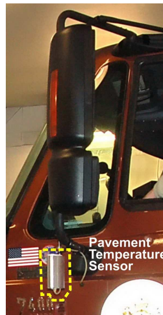
Figure 3. Pavement Temperature Sensor
