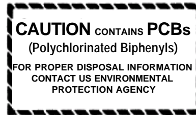
Figure 5-2. Small PCB Mark, also referred to as M_S . The size required by the regulations at §761.45(b) is 1 inch by 2 inches.
