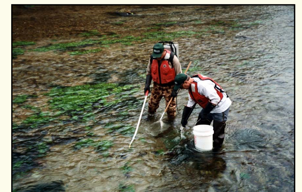
USGS biologists collect fish using backpack electrofishing gear.
