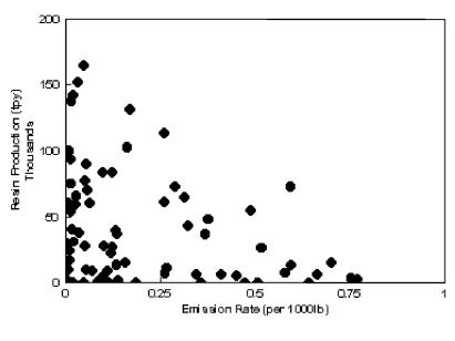
No apparent correlation between the size of the facility and the emission rate for resin production.
