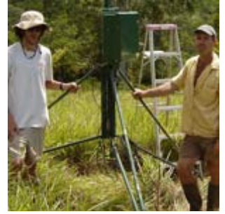
Research staff install a weather station and sensors as part of Hawaii EPSCoR Limahuli Mountain-to-Sea Research. Credit: Courtesy of the National Tropical Botanical Gardens and the Center for Conservation Research & Training, University of Hawaii.
