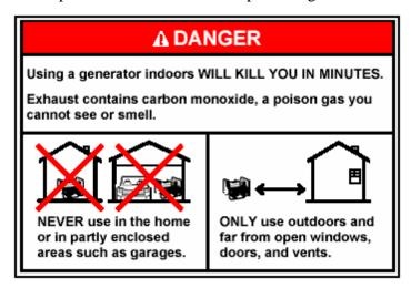
A different representation of the generator may be substituted for accuracy if consumers are likely to recognize it as the generator to which this label is affixed.
