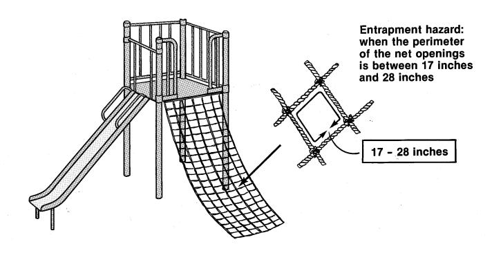
Parents should check for playground cargo nets that could allow head entrapment and strangulations. Net openings should either be too small to permit entry of a child's body or large enough to permit free passage of a child's head.
