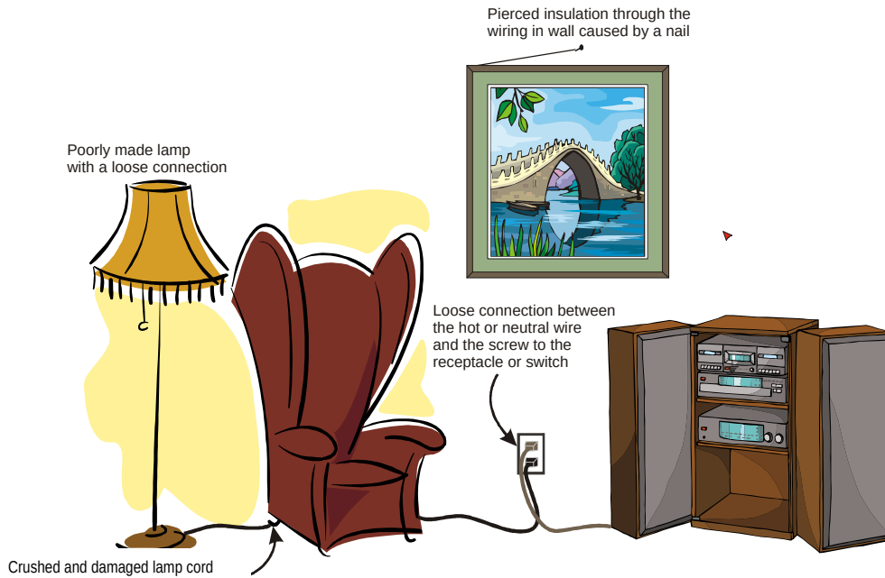
Figure 8. Illustration of Possible Causes of Arc Faults
