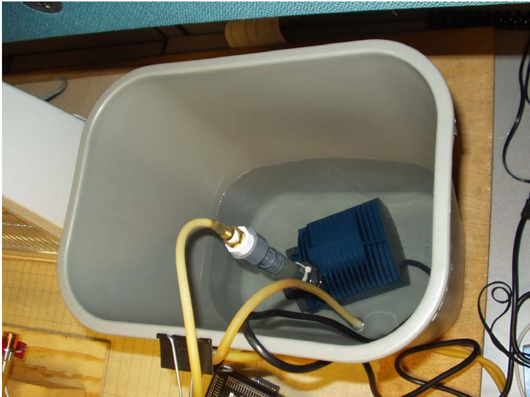
Figure 4: Water Pump and Container
