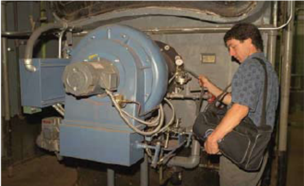
Above: Jamie Harvey uses a Lumex unit to test for mercury at an industrial site. Credit: D. Hansen, Minnesota Pollution Control Agency.
