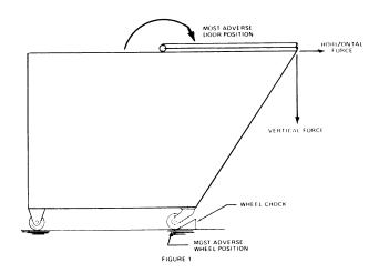
(b) These forces shall be applied separately and the bin shall not tip over under the application of either action cited above in paragraph (a)(1) or (a)(2).
