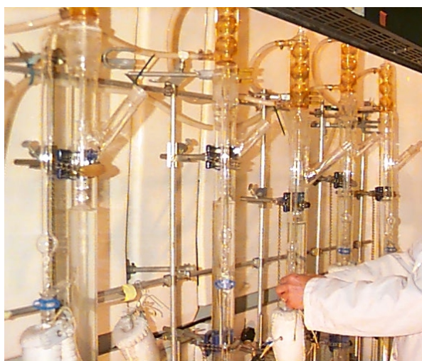
Figure 1. Continuous liquid-liquid extractors with solvent-dispersing frits.
