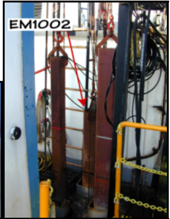
Figure 4. Standpipe of EM1002.
