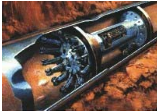
Figure III-4. Illustration of Smart Pig Inside Pipeline
