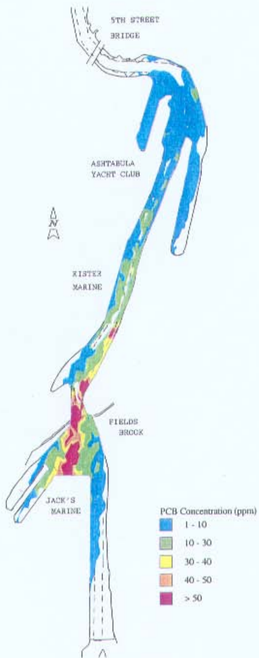
Figure 11: 2D Slice of PCB Plume At -10 feet LWD.
