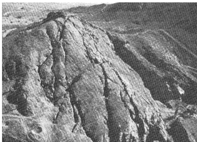
Figure 2. Aerial photograph of open stopes on Mine Hill, Mahd adh Dhahab epizonal vein deposit, Saudi Arabia (from Hilpert et al. 1984). The stopes outline a “tensile-shear” fault mesh within an extensional stepover between left-lateral strike-slip faults. Extensional faults strike towards the top of the photograph and are segmented by oblique, synthetic and antithetic shear faults. The segmentation imparts the observed zigzag pattern of the stopes.
