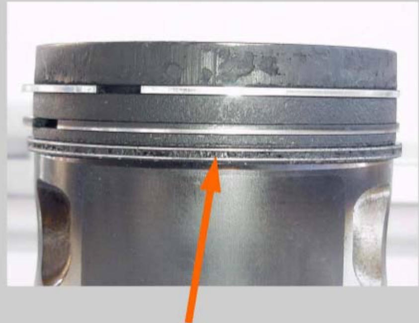
Deposit forming in the piston ring area
