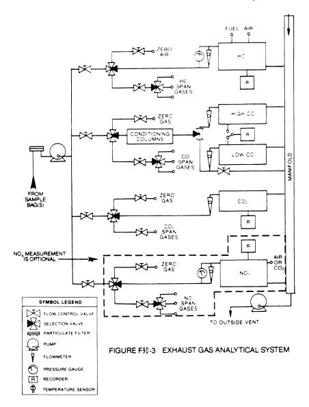
(b) Major component description. The exhaust gas analytical system for HC, CO and CO<sub>2</sub>, Figure F90–3, consists of a flame ionization detector (FID) (heated  $(235^{\circ}\pm15~^{\circ}\text{C}~(113^{\circ}\pm8~^{\circ}\text{C}))$  for methanol-fueled vehicles) for the determination of hydrocarbons, nondispersive infrared analyzers (NDIR) for the determination of carbon monoxide and carbon dioxide
