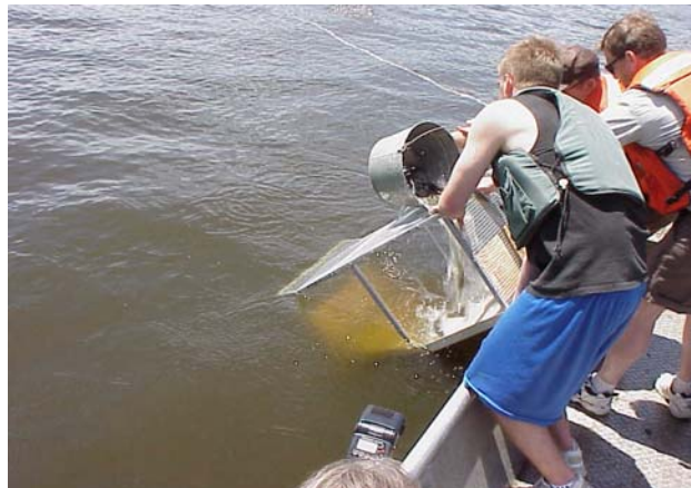
Figure 11. Cages used to propagate Higgins' eye pearlymussels on the Upper Mississippi River. Cages are constructed of aluminum sides, base and ½-inch screen. The top left photo shows two types of cages; the cage on the left is used in low current areas and the right one in higher velocity areas. These are open cages with no bottoms; closed cages have a 3/8-inch plywood bottom to collect transformed mussels (top right photo). The middle and bottom photos show the process of transporting cages (closed) to the relocation site, adding host fish (smallmouth bass) and placing cages on the river bottom. (photos courtesy of the Minnesota Department of Natural Resources and U.S. Fish and Wildlife Service)
