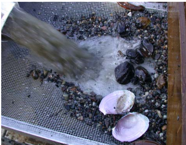
Figure 13. Suction dredge used by the Minnesota Department of Natural Resources to sample mussels. Diver places suction nozzle inside cage or on river bottom; contents are pumped to screening trays where mussels are sorted. (photos courtesy of the U.S. Fish and Wildlife Service)
