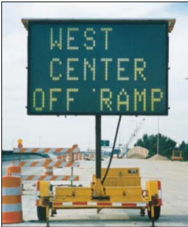
West Center off-ramp variable message sign
