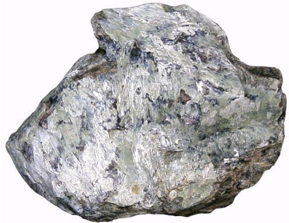
A serpentinite sample dominated by lizardite, a mineral that gives the rock a soft, soapy feel.
