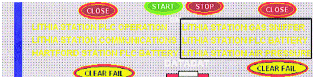
Figure 4.7. Light background with light colored foreground makes reading yellow text in center of display difficult. The yellow text shows alarms such as a battery alarm in the black rectangle above.
