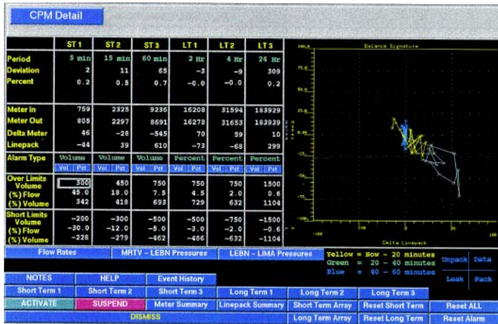
Figure 4.15. CPM Screen with values on the left of the screen to indicate over six time periods (three short term indicated by ST and three long term indicated by LT). On the right of the screen are three lines graphically depicting possible leaks over three time periods.
