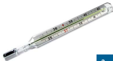
Examples of a mercury thermometer (a) and an alcohol thermometer (b).
