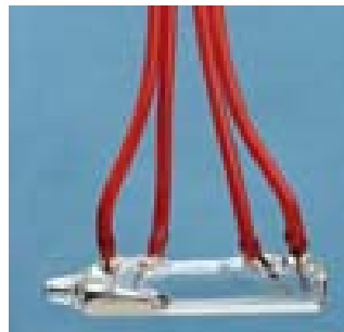
Example of a mercury electrical switch. Notice the pool of silver-colored elemental mercury on the left side of the switch.
