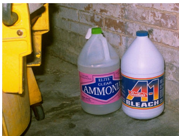
Example of incompatible chemical storage: when bleach and ammonia are mixed together, toxic fumes of chlorine gas are released.
