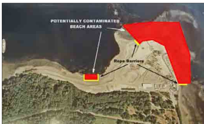
Potentially contaminated beach areas and rope barriers.
