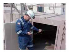
Because of the poor airflow toxic gases can accumulate in a confined space. Before any miner enters a confined space, the air needs to be checked for adequate oxygen concentration and the accumulation of flammable gases. Many electronic instruments have remote sampling probes so that a miner Can sample the atmosphere in a confined space from a safe location. Only after the atmosphere is judged to be safe should miners enter the confined space.
