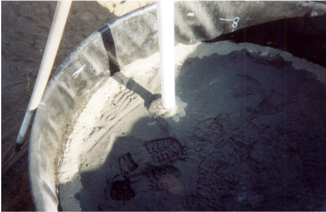
Figure 4-5. Bentonite beads around test cell outer edge and well pipe.
