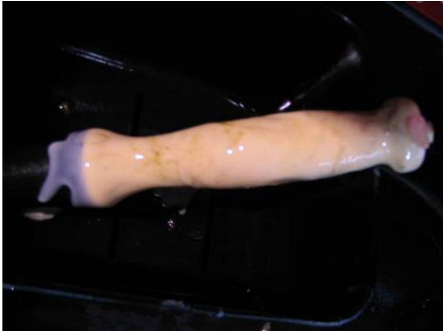
Figure 4. Handle After Exposure to Eagle Kleen III
