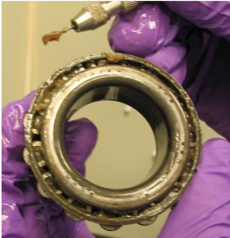
Figure 1. Bearing Inspection after Initial Immersion
