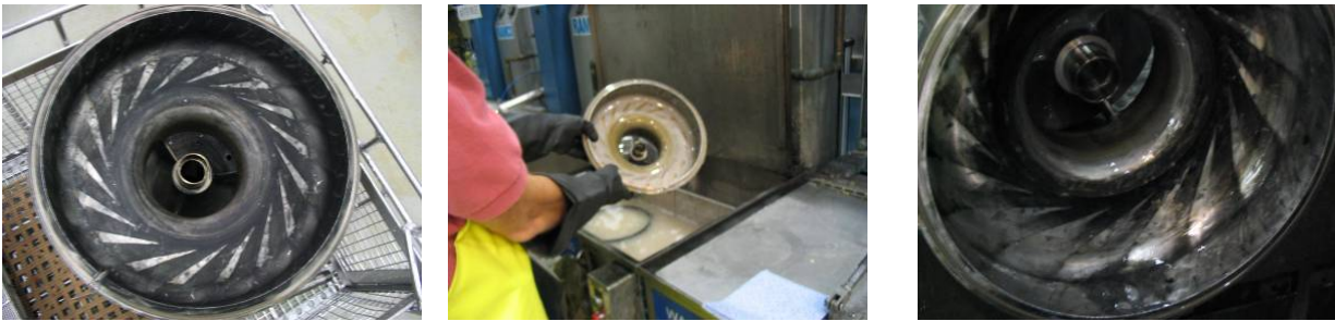
Figure 12. Example of Air Inlet Housing Prior to Cleaning (left), After Degreasing with Turco 6849 (center), and After Degreasing with Eagle Kleen™ (right)
