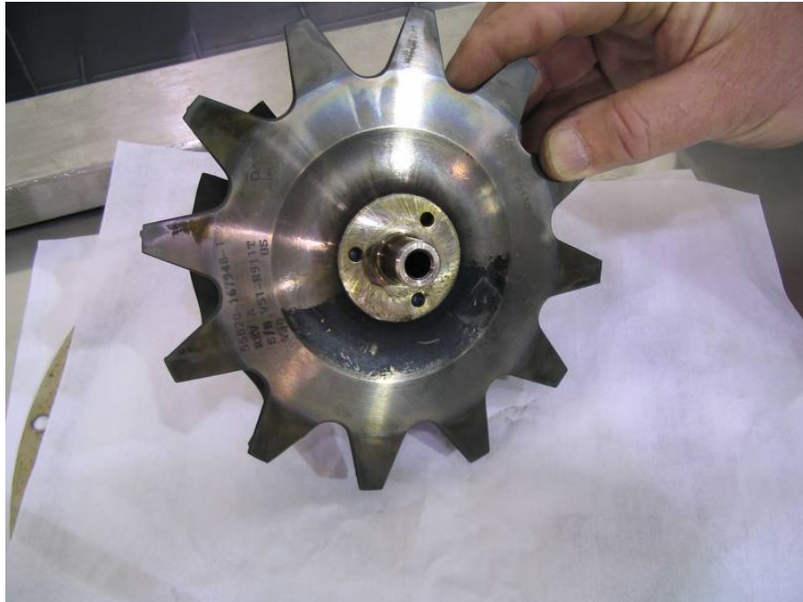
Figure 19. Front View of Fan Assembly after Cleaning
