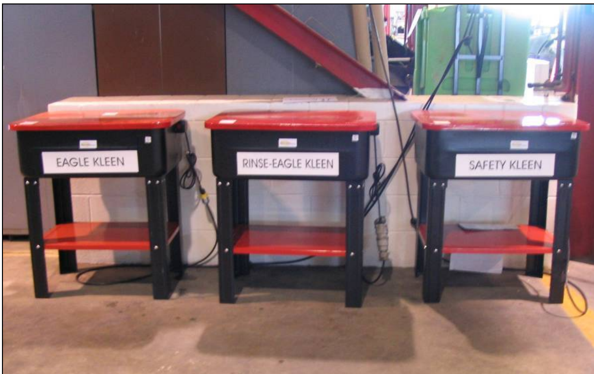
Figure 5. Degreaser and Rinse Tanks for Eagle Kleen™ and Safety Kleen™ Bath
