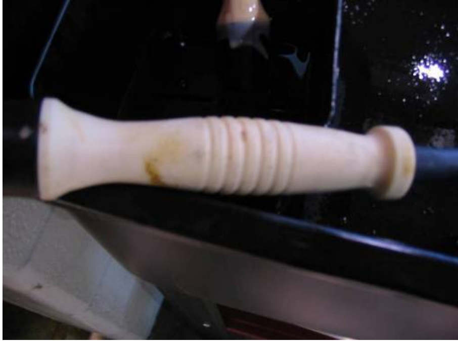
Figure 3. Handle Before Exposure to Eagle Kleen III
