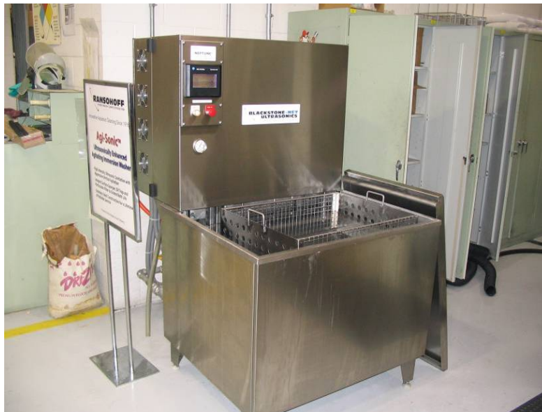
Figure 21. Agisonic AG-30 Shown from Front (Note: the lid is set off to the right of the tank)
